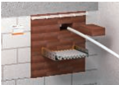
Simple reinstallation through removal of individual blocks
