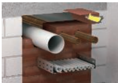
Running of combustible pipes without additional measures
