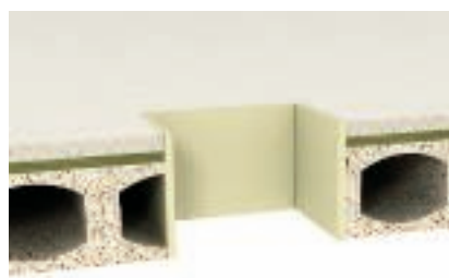
Cavity chamber ceiling
